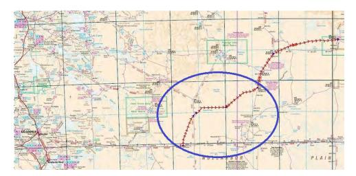
From approximately 100kms west of Red Drum Corner to just prior to Red Drum Corner is in very bad condition with poor soil and many blow outs. This portion of road is in the City of Kalgoorlie-Boulder but is not on their road inventory.
